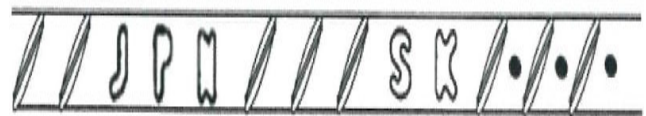
(JPN9) SANKO SEIKO CO., LTD. (●) mark / marks may be found on the same / opposite side of the bar at random
